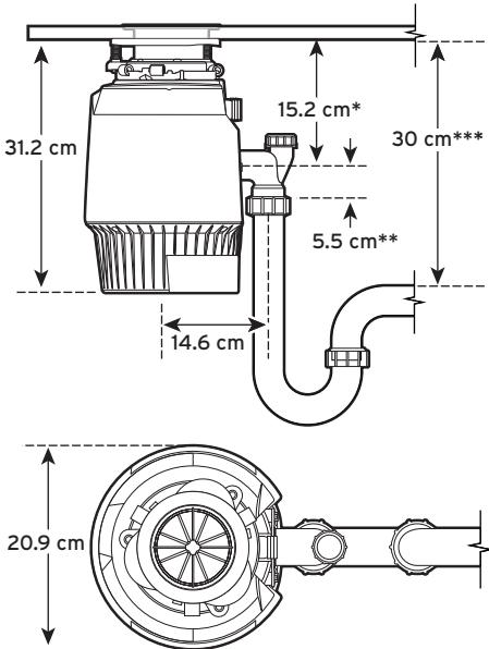
\*Distance from bottom of sink to centre line of disposer outlet.
